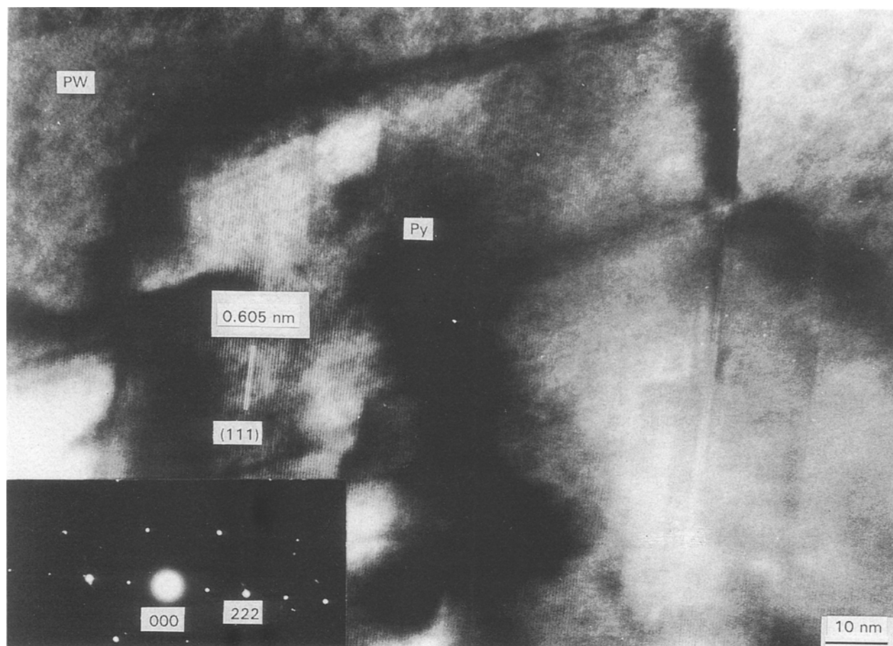
Figure 3 High-resolution electron micrograph of Py phase in a sample prepared at 910 °C, 58 h.
